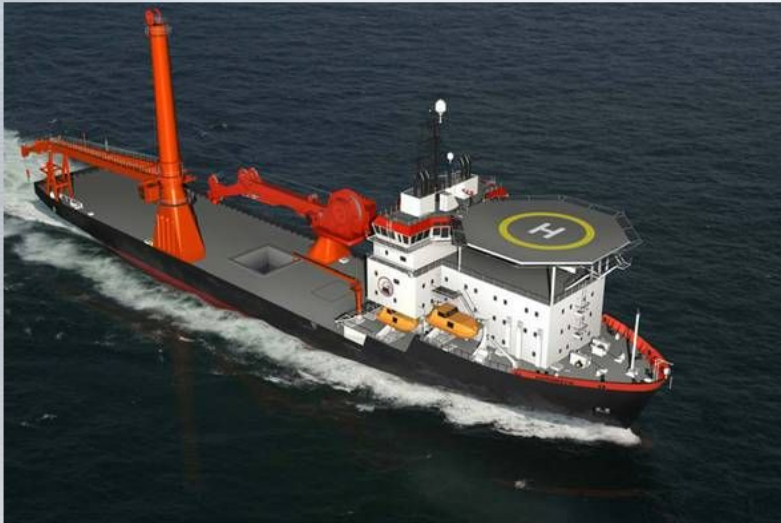
(Hornbeck TBN – Merwede Type 22 design – DP3 multipurpose construction vessel)
